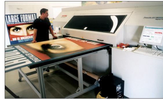
The PressVU at the Weger GmbH printed in 8 colour-mode with activated smooting-function, which eliminated Banding, but also slowed down the process. The upper image shows production manager Tim Bangert.
